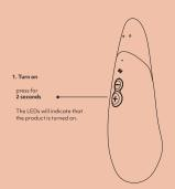
1. Turn on / off A haptic feedback (short vibration) and the LED will indicate that the product is turned on.
